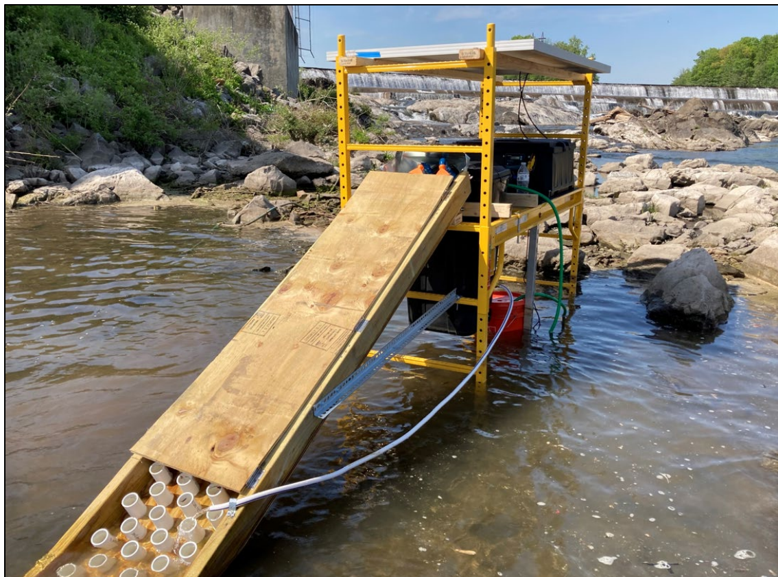
Figure 2-1: Eel Ramp Trap Installed Downstream of the Crescent Dam Tailrace Area (Crescent Trap #1).
