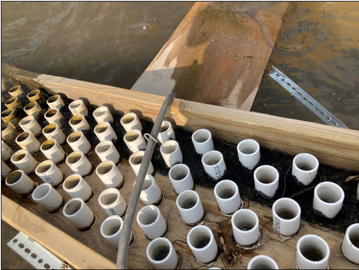
Figure 2-2: Eel Ramp Trap Climbing Substrate with Encamat®
