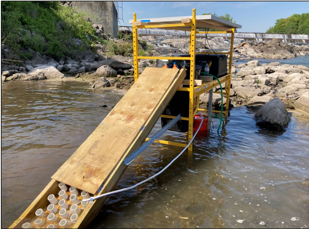
Figure 4-19 Eel ramp trap installed at downstream of the Crescent Dam tailrace area (Crescent Trap #1)
