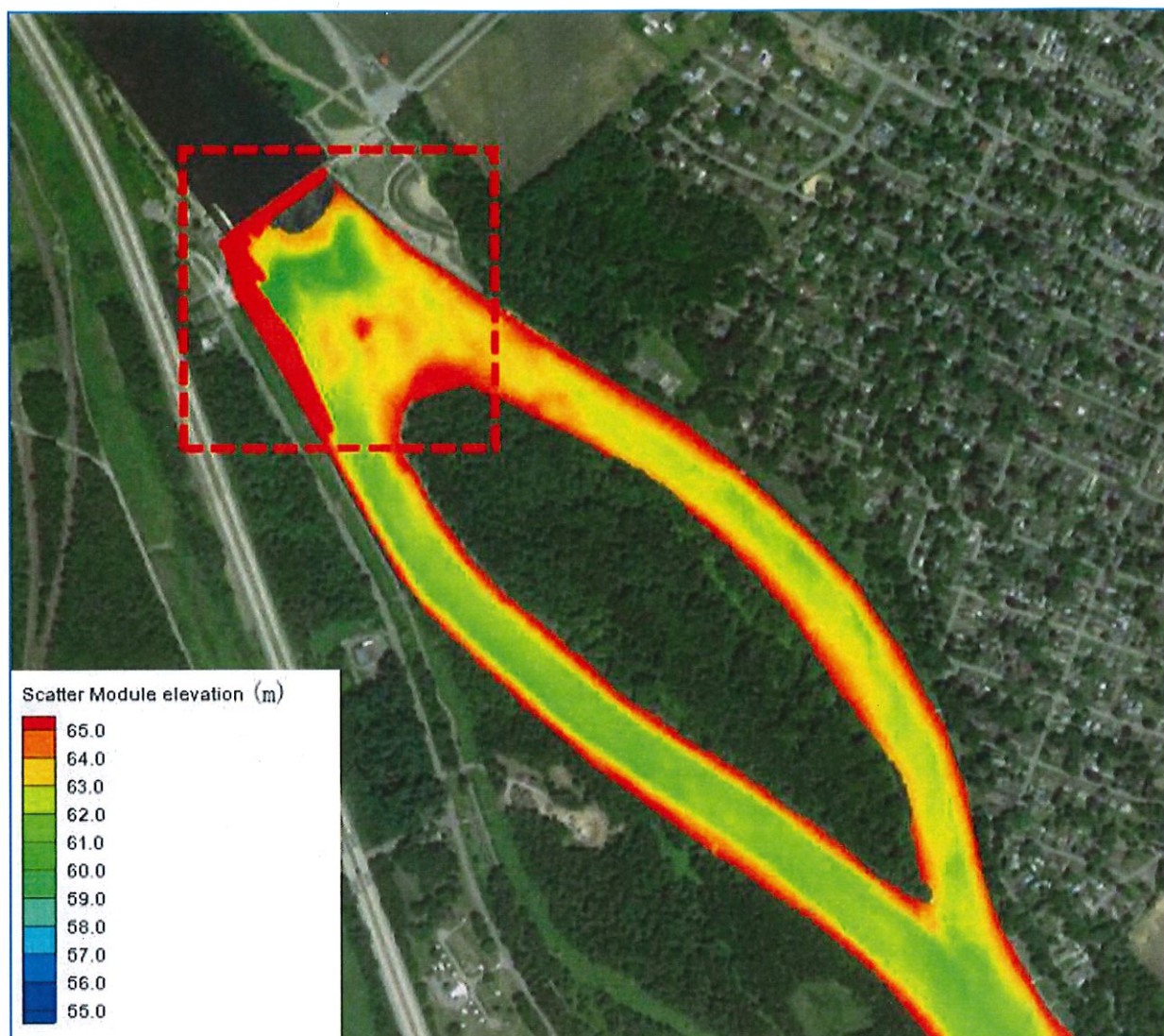
Figure 8: August 2019 Bathymetric Survey of Isle of the Oneidas (outside Schenectady), showing sedimentation and a narrowed river channel
